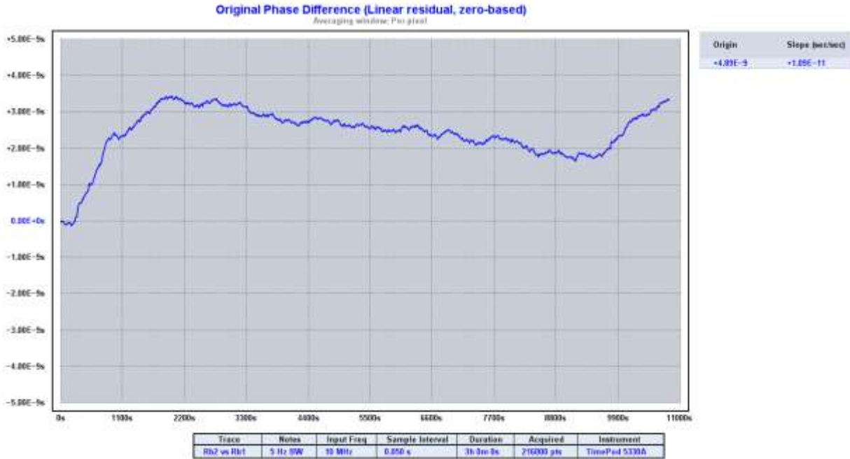
Figure 12. Phase Residuals for Two Rb Oscillators
