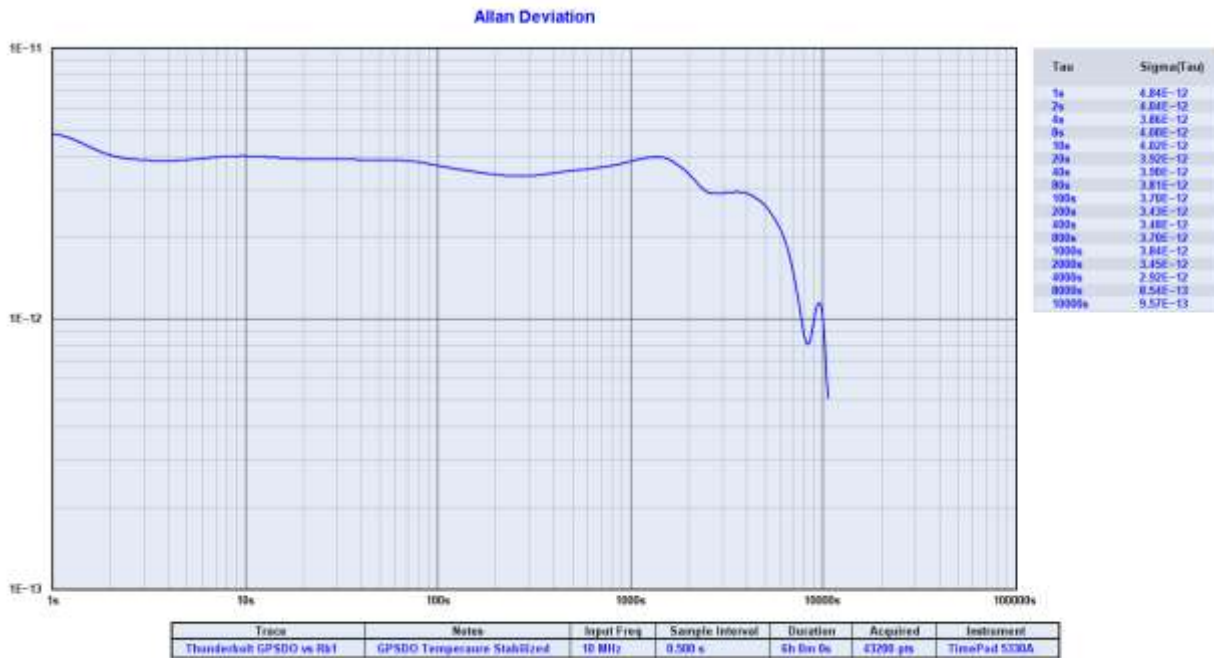
Figure 22. GPSDO versus Rb1 Stability Plot
