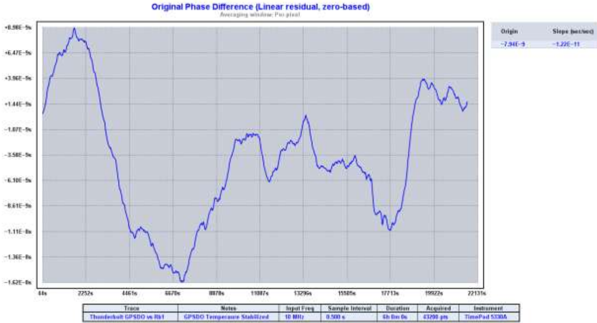
Figure 19. GPSDO versus Rb1Phase Residuals Plot
