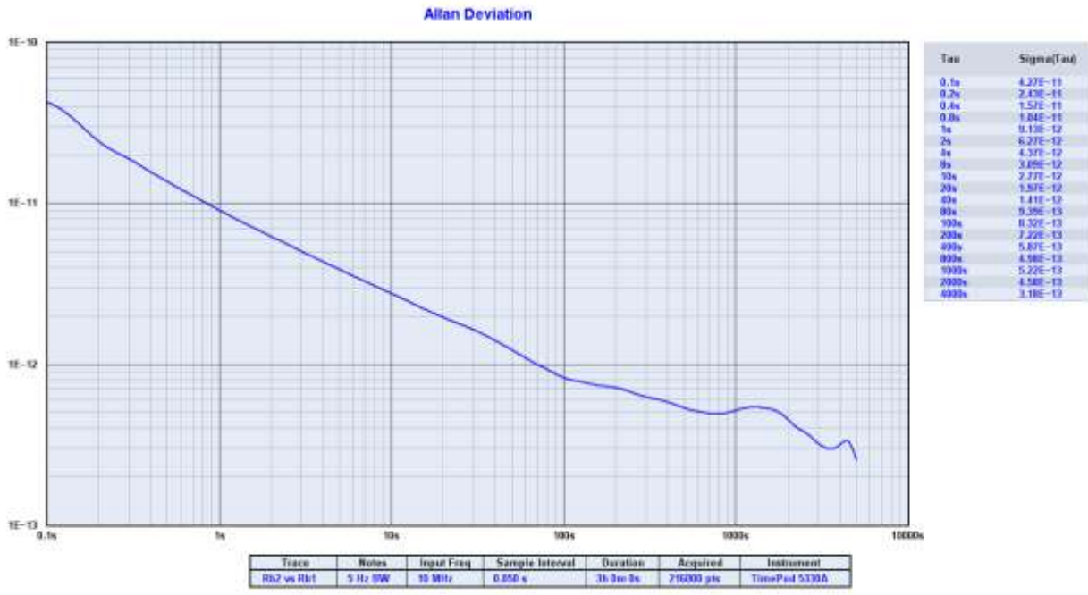
Figure 14. Frequency Stability Plot for Two Rb Oscillators
